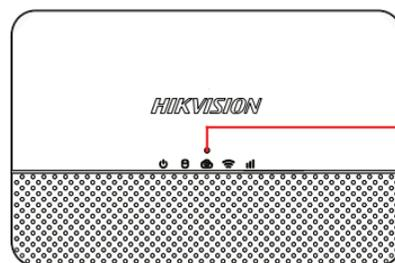
Power on the device, and wait for about 1 min. If indicator
