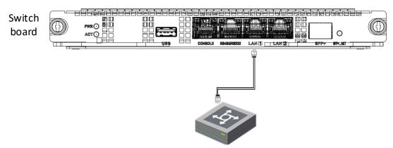
Figure 2-7 Switch Board Network Connection
