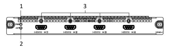
Figure 1-10 Front View of HDMI Input Board
