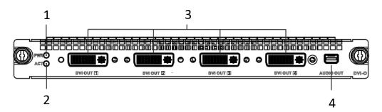
Figure 1-9 Front View of DVI Output Board
