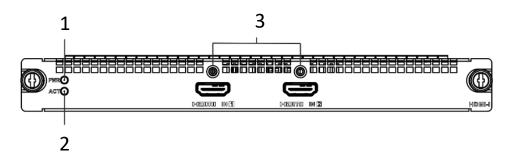
Figure 1-6 Front View of HDMI UHD Input Board
