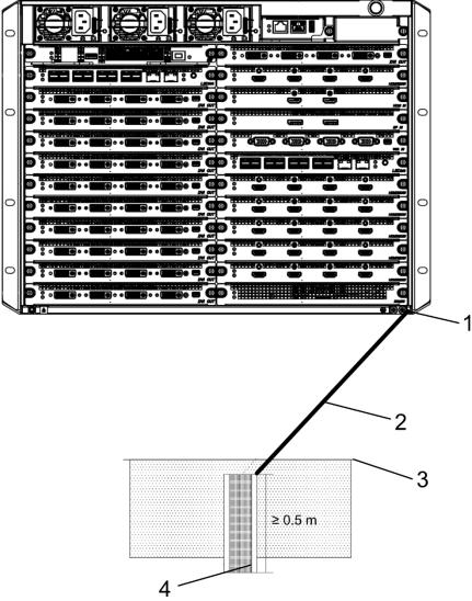
Figure 2-6 Connect the Grounding Cable to the Ground
