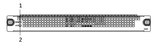
Figure 1-13 Front View of Network Decoding Board
