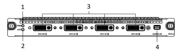
Figure 1-8 Front View of DVI Input Board
