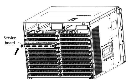
Figure 2-2 Insert a Service Board
