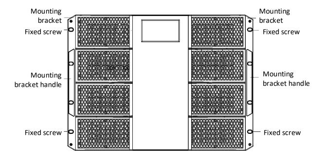
Figure 2-4 Rack Mount the 8 U Device
