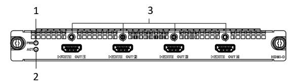
Figure 1-11 Front View of HDMI Output Board
