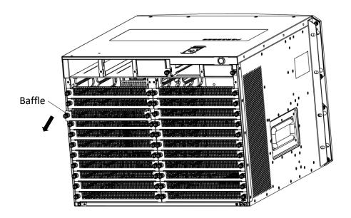
Figure 2-1 Remove the Baffle
