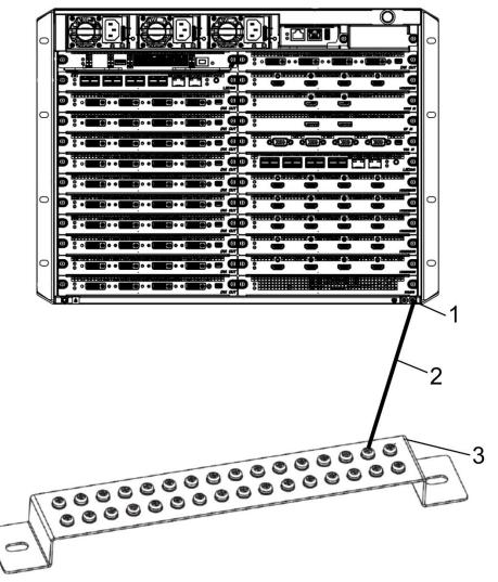
Figure 2-5 Connect the Grounding Cable to the Grounding Row
