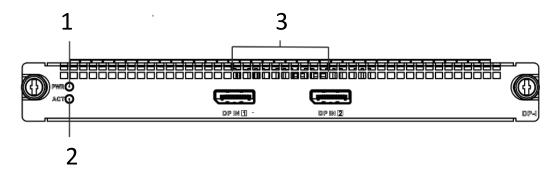
Figure 1-7 Front View of DP Input Board
